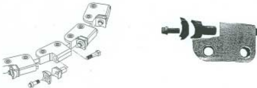
FIG. 16 COMBINATION NO. 2: GILBERT ROUND BACK TOOTH WITH FLAT BACK ADAPTER ON QUADCO TOOTH HOLDER (EXHIBITS P-104 AND P-105)
