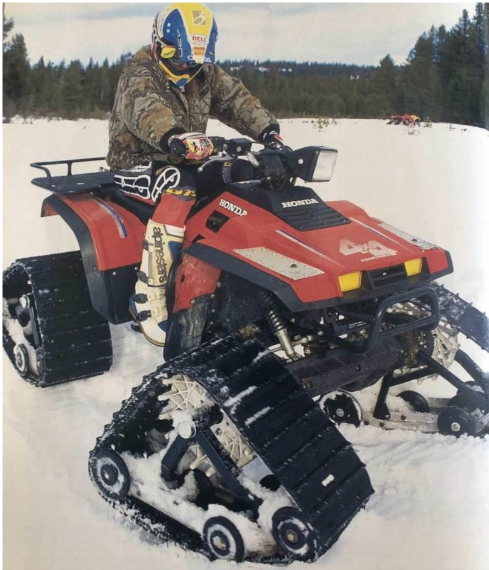
ATV with Quad-Traxx conversion kit installed
