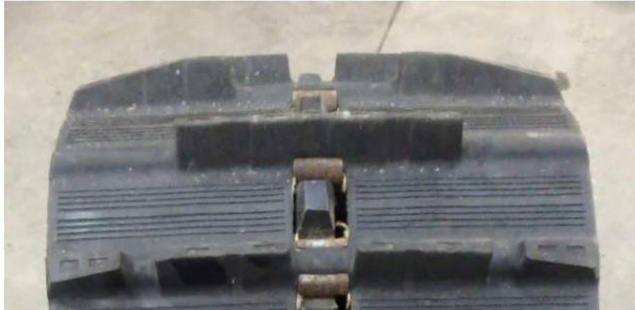
Profile of traction projections (Tatou 2)
