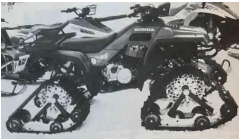
ATV with Quad-Traxx conversion kit installed (side view)
